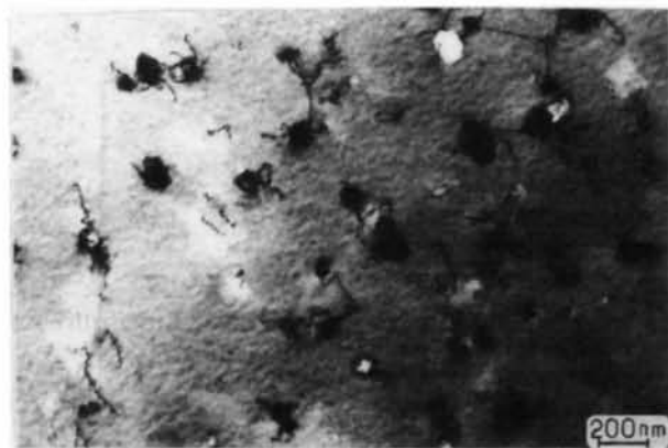
Fig. 8. Microstructure of the Cu-2 at.% Co alloy aged at 923 K for 120 h.
